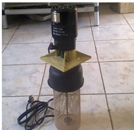
1-Rotating shaft. 2- Epoxy 3-impeller. 4- Motor
