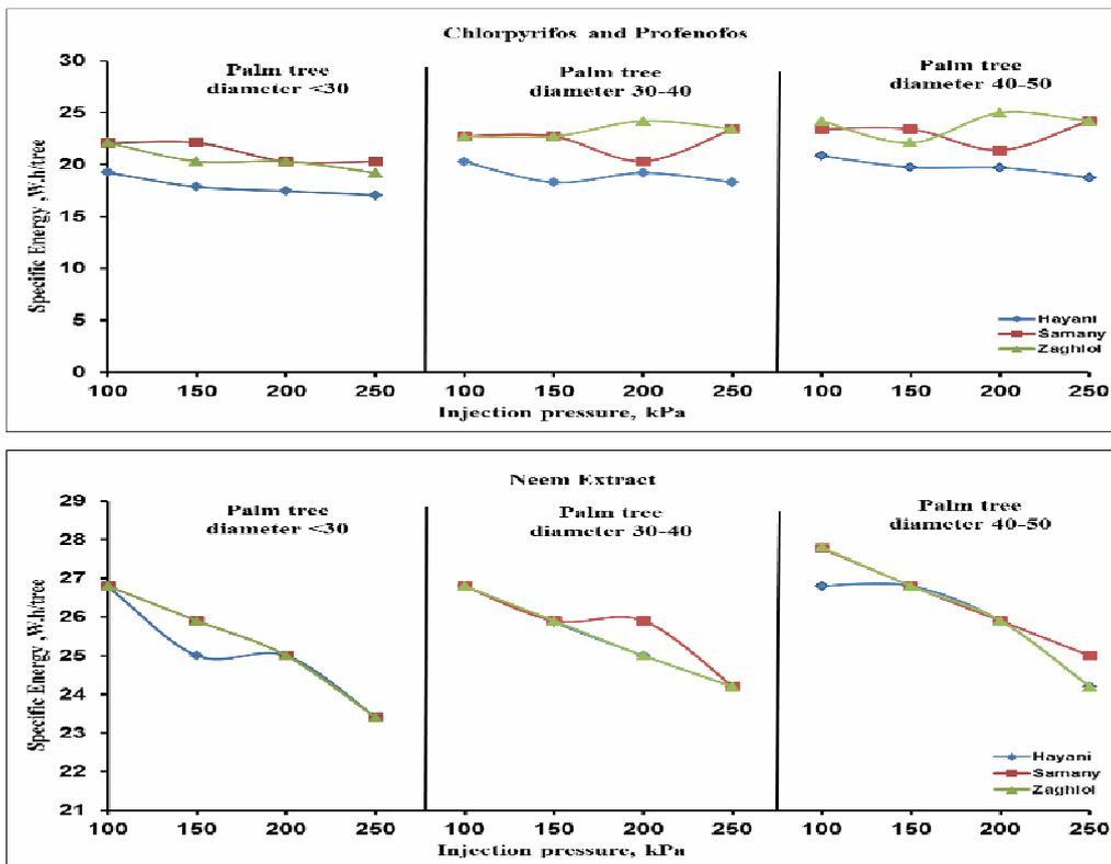
Fig. 8. Effect of injection pressure on specific energy under palm tree diameters and varieties by using chlorpyrifos, profenofos insecticides and Neem extract
