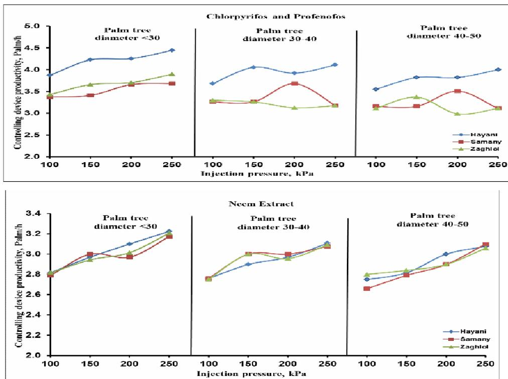
Fig. 6. Effect of injection pressure on controlling device productivity under palm tree diameters and varieties by using chlorpyrifos, profenofos insecticides and Neem extract
