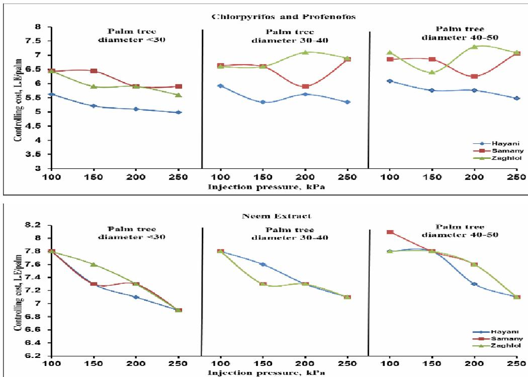
Fig. 9. Effect of injection pressure on controlling cost under palm tree diameters and varieties by using chlorpyrifos, profenofos insecticides and Neem extract
