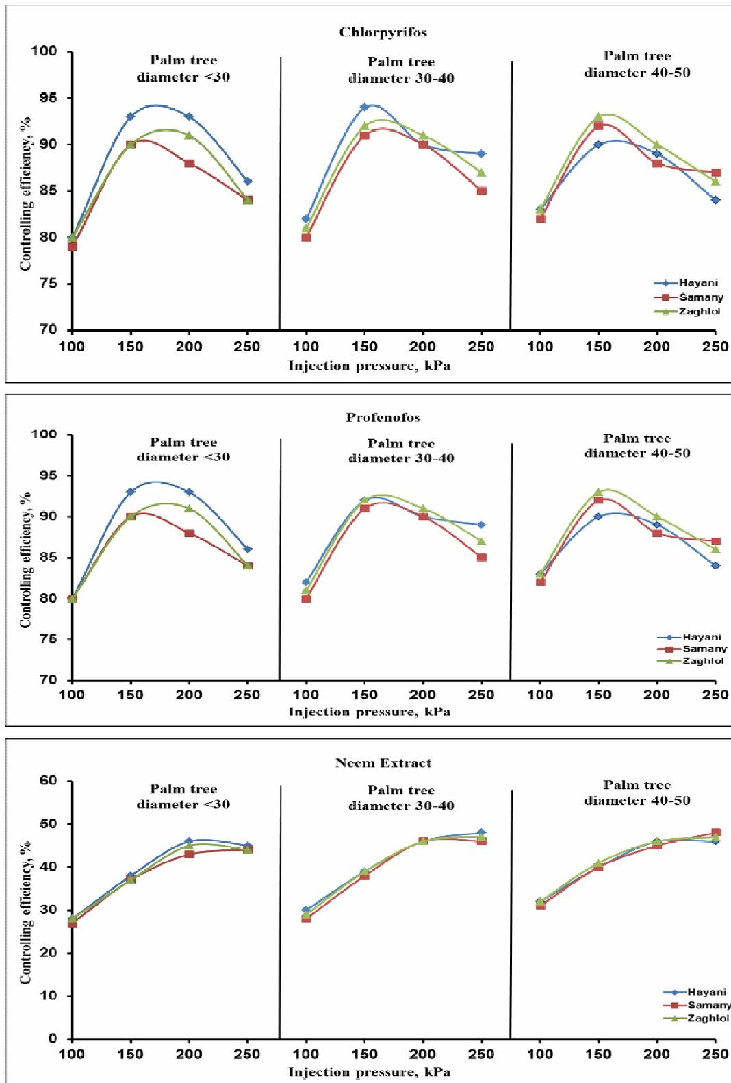
Fig. 7. Effect of injection pressure on controlling efficiency under palm tree diameters and varieties by using chlorpyrifos, profenofos insecticides and Neem extract
