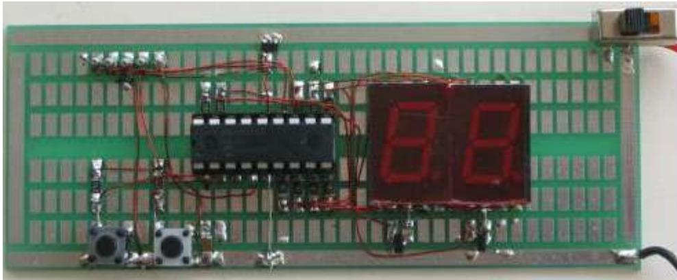
**Fig. 4.** Photograph of the up counter circuit
