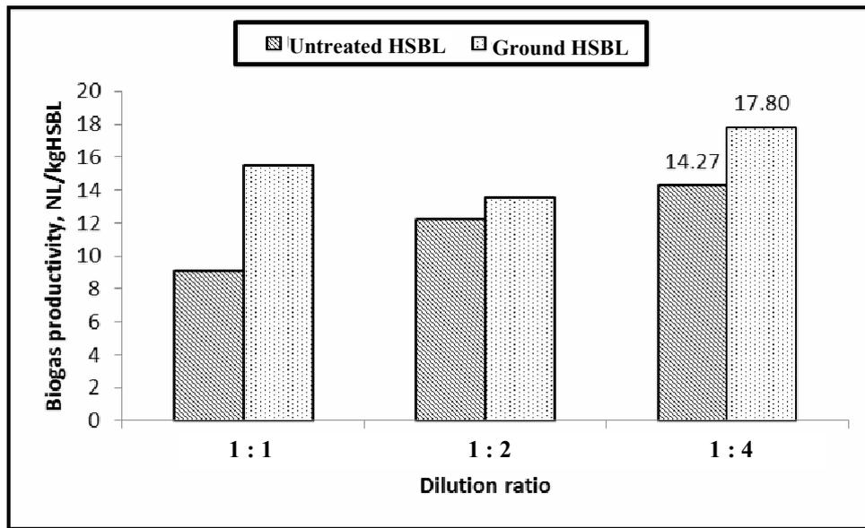
Fig. 2. Biogas productivity from dry AD of untreated and ground HSBL with respect to mass of HSBL in the content of reactor
