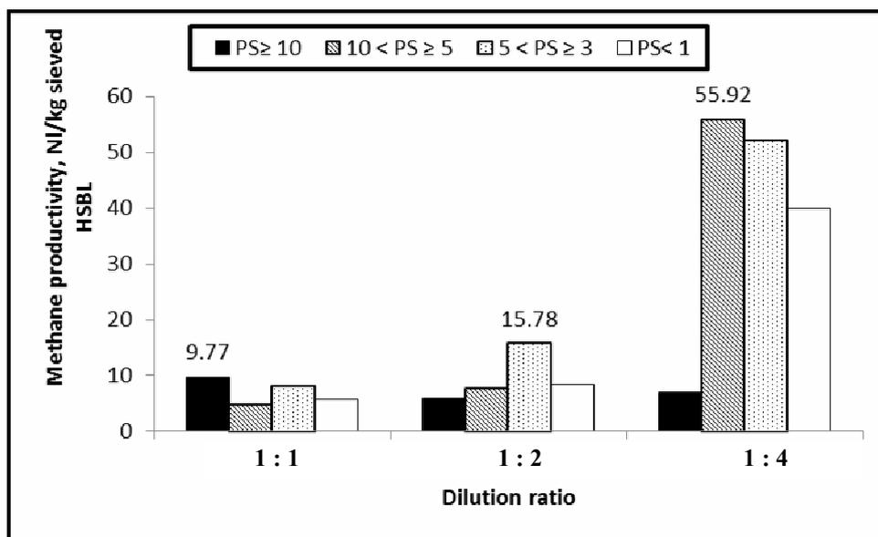
Fig. 5. Methane productivity from dry AD of sieved HSBL with respect to mass of sieved HSBL in the content of reactor
