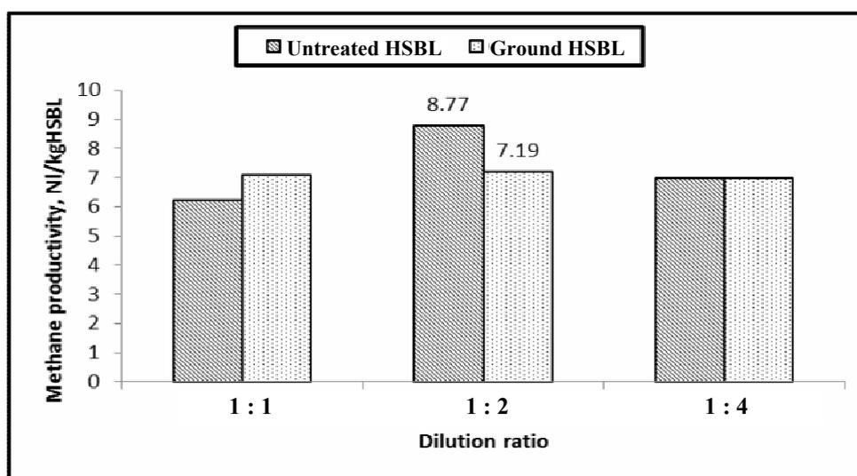
**Fig. 4. Methane productivity from dry AD of untreated and ground HSBL with respect to mass of HSBL in the content of reactor**
