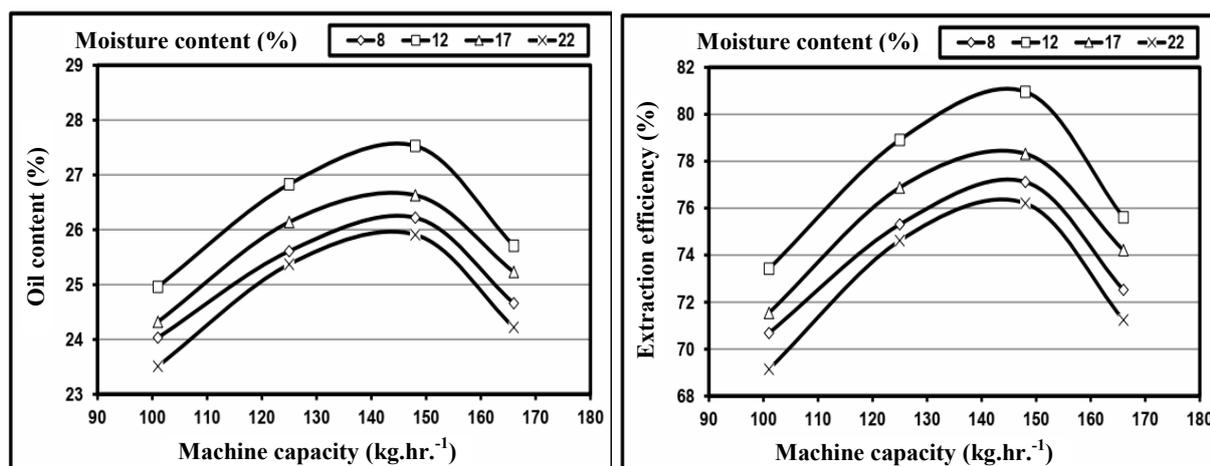
Fig. 3. Effect of machine capacity on oil content and extraction efficiency
