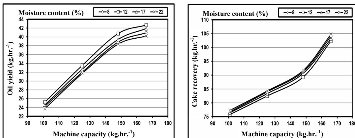
Fig. 4. Effect of machine capacity on the oil yield and cake recovery
