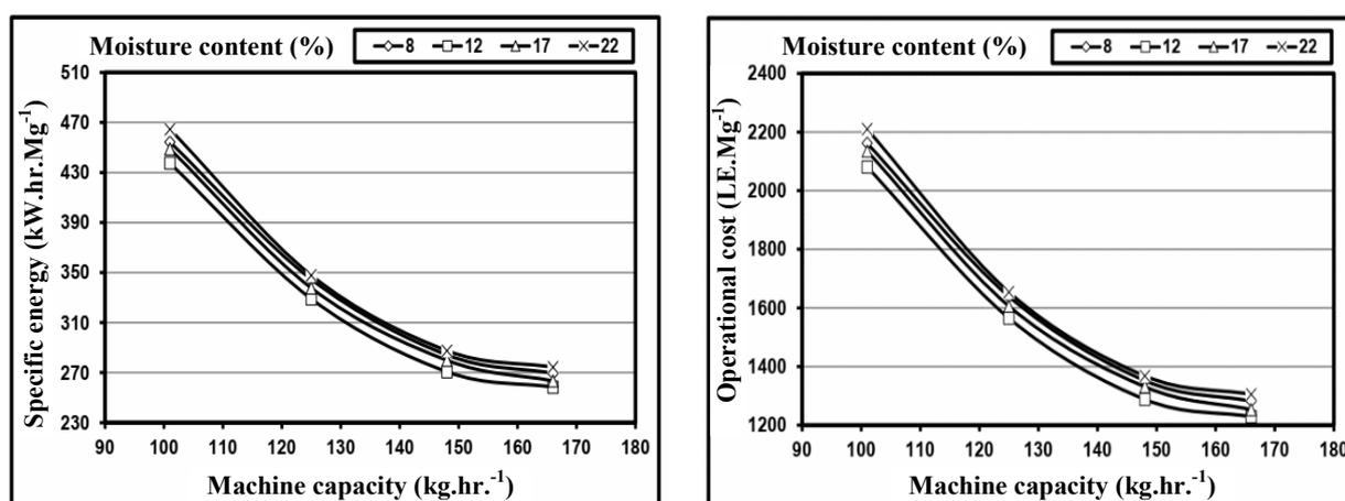
Fig. 5. Effect of machine capacity on specific energy and operational cost
