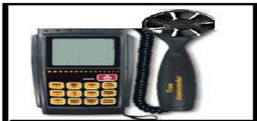
Fig. 3. Device measurement air velocity
