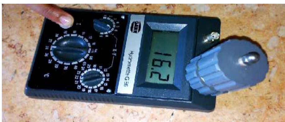
Fig.4. Electronic moisture meter
