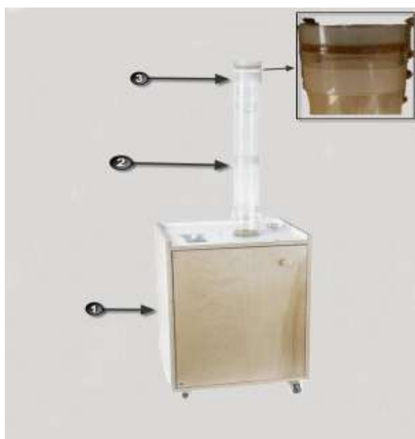
Fig. 1. Terminal velocity device: (1) Wooden box contain blower motor, (2) Column constructed of clear Plexiglas, (3) Calibrated valve cap
