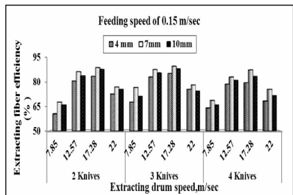
Fig. 4. Effect of extracting drum speed on sisal fiber productivity under different clearances, and knife number using feeding speeds of 0.05, 0.1 and 0.15 m/sec.
